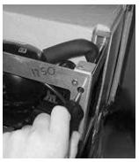
8. After you lift the cabinet off the frame you can service the agitator motor.
